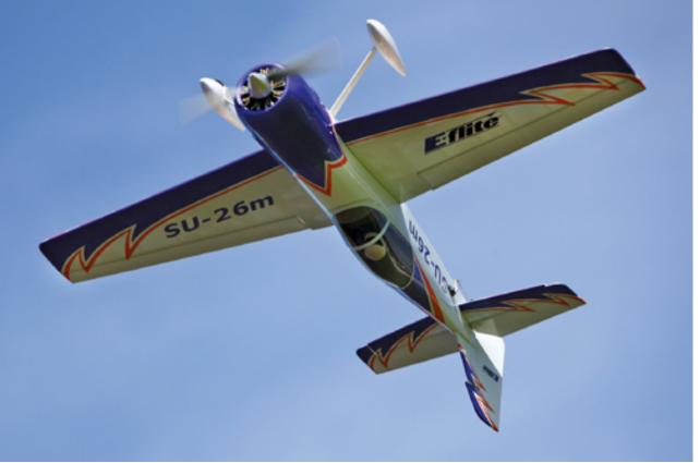
In the early days of aviation, spins were often fatal because most pilots did not understand how to properly recover from a spin. While in an upright spin, the pilot would pull back on the elevator stick in an effort to save the airplane (and their life!) and only make the situation worse. Since the spin occurs when the aircraft is in a stalled state, adding elevator just keeps the airplane stalled.
